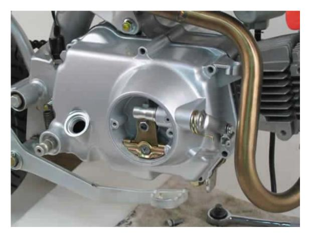
C27. Install a new seal over the kick-start lever.
