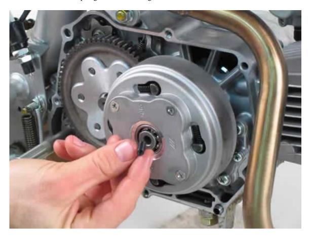
C23. Install the new oil passage tube over the spring and into the bushing.
