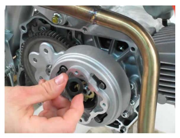
**C18**. Install the new retaining nut. Use a strap wrench and a clutch nut tool to tighten the retaining nut to 31 ft-lb. After the retaining nut has been tightened down, use a small flat blade screwdriver to bend the arms of the lock washer into place.
