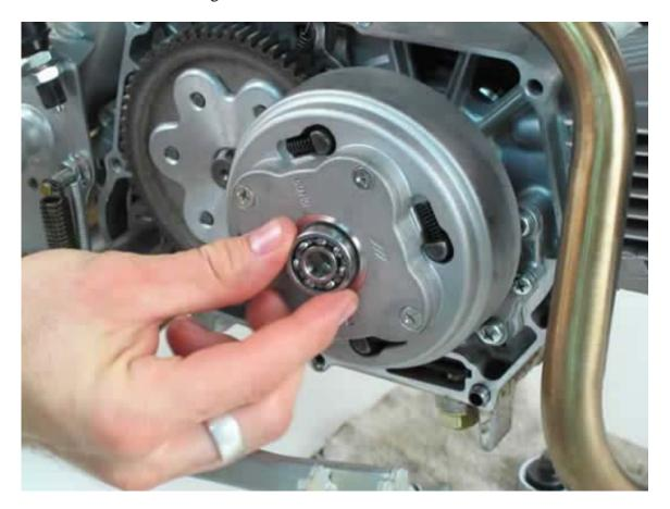
C21. Install the new oil passage bushing into the bearing.
