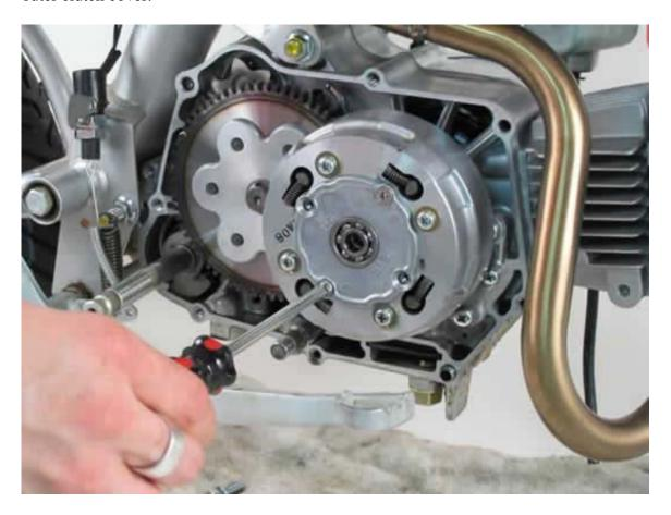
**C4.** Use a small flat blade screwdriver and open up the tabs on the lock washer. Use a clutch nut tool and a strap wrench to remove the black retaining nut. Remove the clutch assembly.
