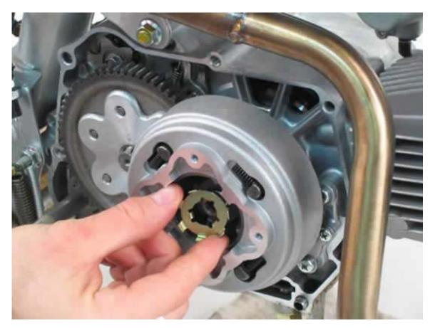
C17. Install the new cup washer. Make sure that the tapered end of the washer faces away from the engine.
