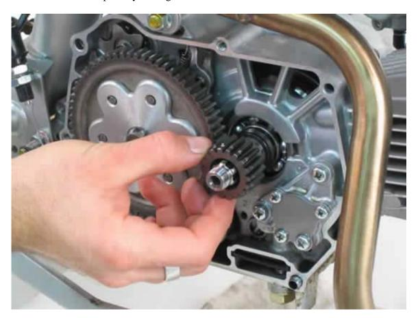
**C16**. Install the new clutch assembly. Note that the backside of the clutch assembly locks onto the primary gear. Make sure that the clutch assembly is locked into place before proceeding. Install the new lock washer.
