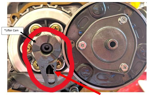
26. Install the clutch lever/arm. It must land here on the lifer cam.
