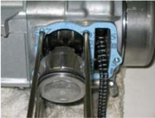
9. Install a small black seal into the lower hole.
