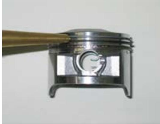
5. Lightly coat the wrist pin with clean motor oil.
