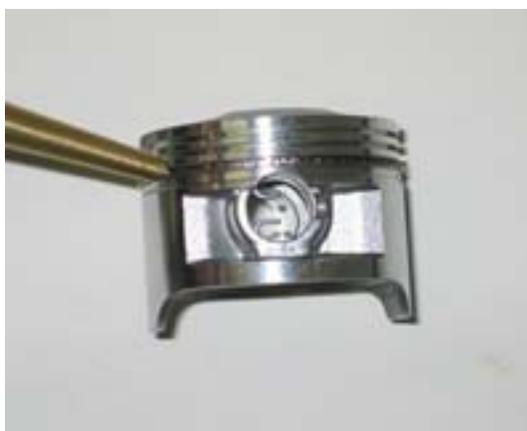
4. Install the lower piston ring (which is flat black in color) onto the lower groove in the piston. After the lower ring has been installed, install the upper ring, which is shiny in appearance. Note that the gap opening on each ring faces the opposite direction.
