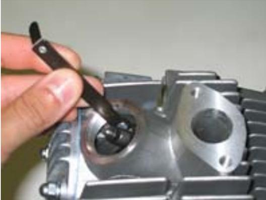
3. After the valve clearance has been set, grab the flywheel and turn the engine over counterclockwise TWICE and re check the valve clearance. If you have done everything correctly, there should be NO gap clearance. If there is a gap, you will need to repeat this step until no gap is present.
