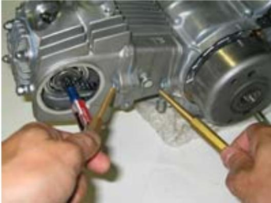
At this point you are now ready to install the cam gear and set the valve clearance. Before installing the cam gear, double check that the engine is at top dead center by lining up the "T" on the flywheel with the notch on the engine case. Once the "T" is lined up, look into the spark plug hole with a flashlight and you should be able to see the top of the piston. If everything checks out, then do the following:
