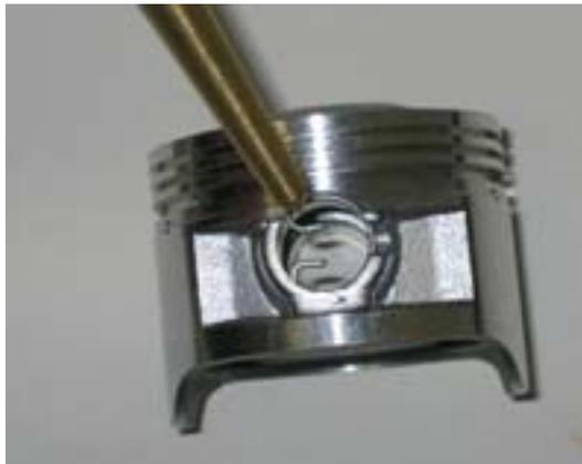
3. Install the thin retaining rings and the wavy oil ring onto the bottom of groove on the piston. Carefully slide one thin retaining ring on, then the wavy oil ring, and then the other thin retaining ring. Make sure that the gap on each ring faces the opposite direction as shown in the picture.
