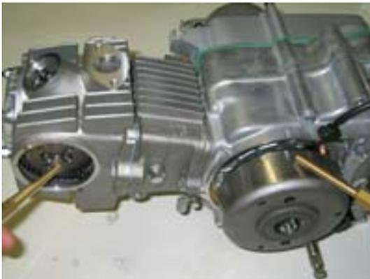
2. Starting with the upper tappet, use a .05mm (.002) feeler gauge to set the valve clearance. Once the gap has been set, tighten the tappet bolt (9mm) to 80 in. lbs. Repeat the process for the lower tappet.
