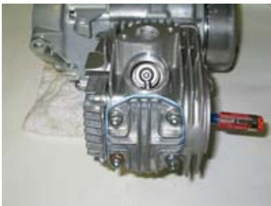
20. Tighten the cam chain roller bolt, the cylinder head side bolt and the cylinder side bolt to 8 ft. lbs.
