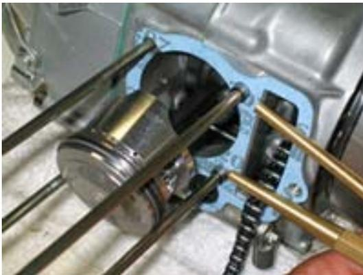
11. Apply a small amount of CLEAN oil into the cylinder and slide the cylinder over the studs. Compress the first piston ring with one hand while CAREFULLY sliding the cylinder over the ring. Do not force the cylinder into place. Repeat the process for each ring until the cylinder is in place.
