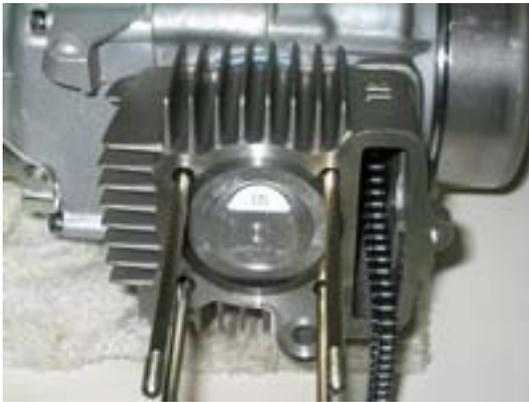
12. Install the black cam chain roller, the cam chain roller bolt (10mm), and the cylinder side bolt (10mm) finger tight.
