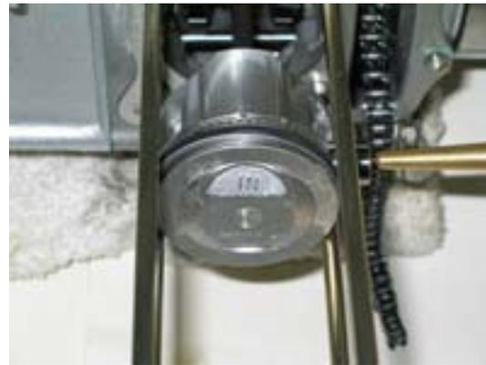
7. Carefully install the second c-clip onto the piston to lock it into place. Once again, compress the c-clip just enough to secure it into the piston. Note the position of the installed c-clip.
