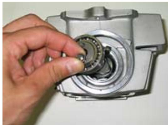
14. Install the new camshaft and make sure that the cam lobes are facing downwards.
