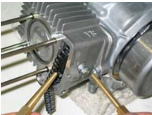
13. Now it's time to remove the camshaft. To remove the old camshaft, loosen the tappets all the way. Lightly screw one of the camshaft gear bolts into the camshaft and pull the camshaft out.
