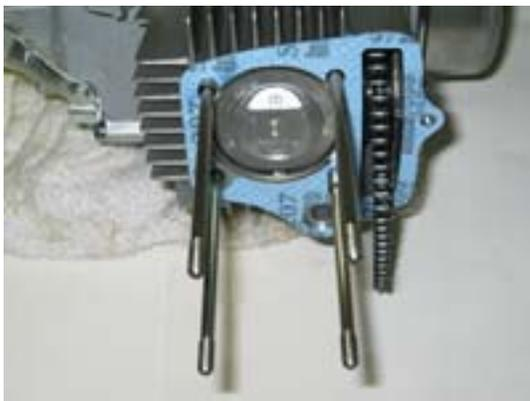
17. Install the green gasket onto the bottom left cylinder stud and place a black gasket into the recessed hole.
