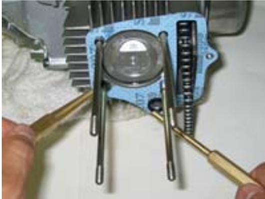
18. Install the cylinder head. Make sure to pull the cam chain all the way through and temporarily lock it into place with a small screwdriver.
